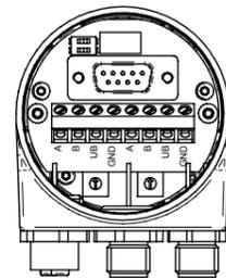
**Terminal assignment for models with additional incremental connector**
